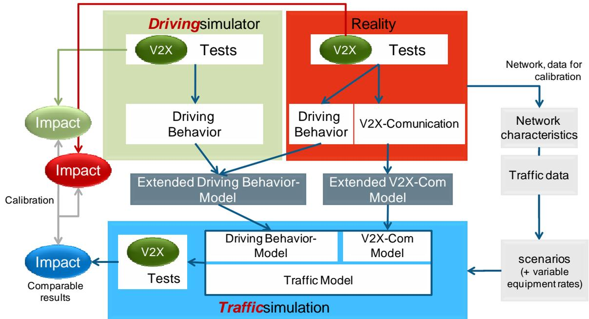
**Fig. 2: Combination and interaction of different test environments (adapted from (1))**
