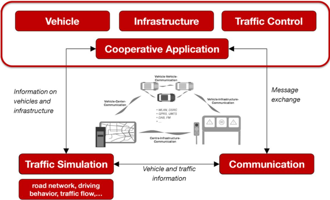
**Fig. 5: Interaction between simulation model, communication model and cooperative application in traffic simulation environment (adapted from (2))**
